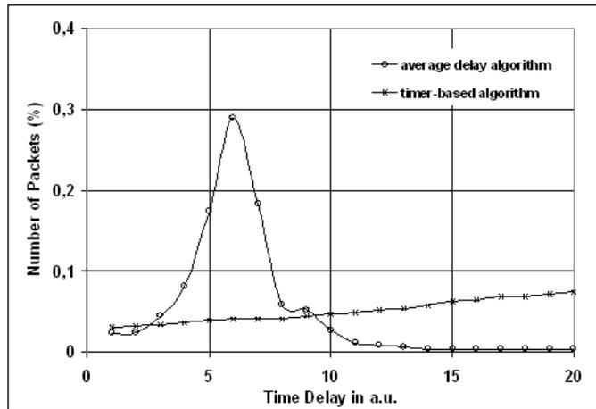
Fig. 4. packet delay distribution for both a timer-based and the proposed average-delay assembly algorithm
